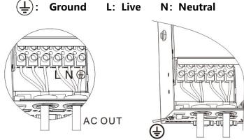
Note: use thick ground cable as far as possible (with cable section not less than 4mm<sup>2</sup>), place the ground point to be close to the all-in-one machine as far as possible and choose shorter ground wire to the greatest extent Wiring method of PV input:
